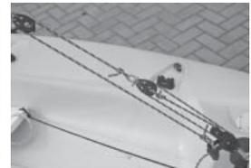
The angle of the cleat should be adjusted to a “fully up” position. This can be changed by unscrewing the center screw and reassembling to the preferred angle. (figure 20)
